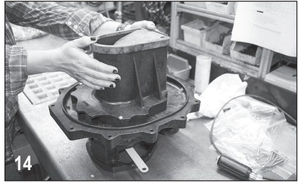
14 Install check valve onto diffuser.
